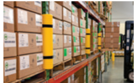
Post guard for pallet rack* Impact guard for attachment to shelving systems
